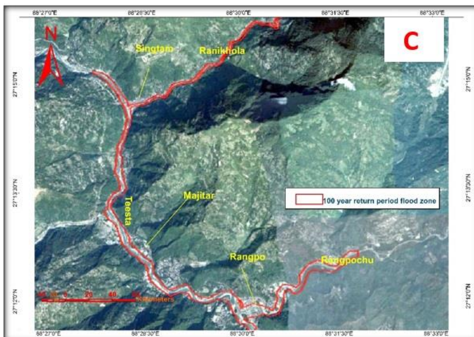
Figure 3.7. (C): Flood zone of 100-year return period flood in the selected stretches of the Teesta, Ranikhola and Rangpochu
