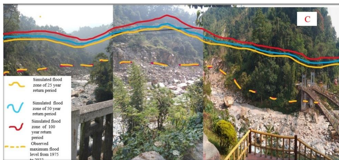
Figure 3.16. (A): Simulated flood zone of 25, 50 and 100-year return period flood at Legship Bazar area. (B) and (C): Observed maximum flood zone at Legship bazar area (1975 to 2021).
