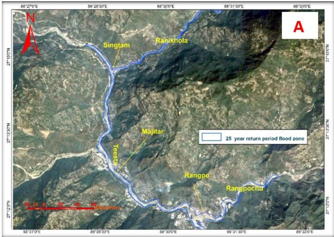
Figure. 3.7 (A): Flood zone of 25year return period flood in the selected stretches of the Teesta, Ranikhola and Rangpochu
