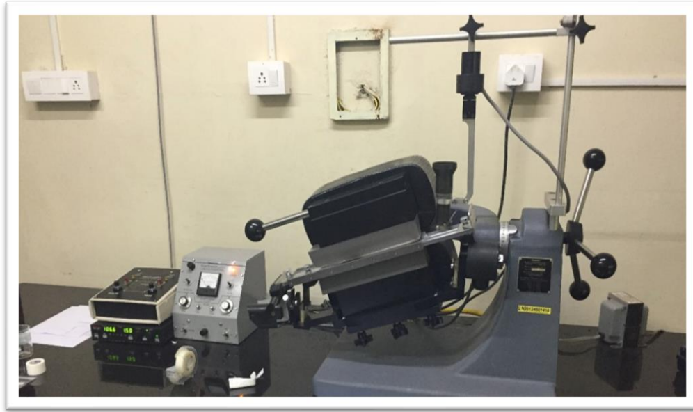
Figure 1.9. Frantz Isodynamic Separator used for separating magnetic and non-magnetic minerals.
