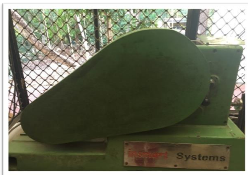
Figure 1.4. Jaw crusher machine for the reduction of sample size.
