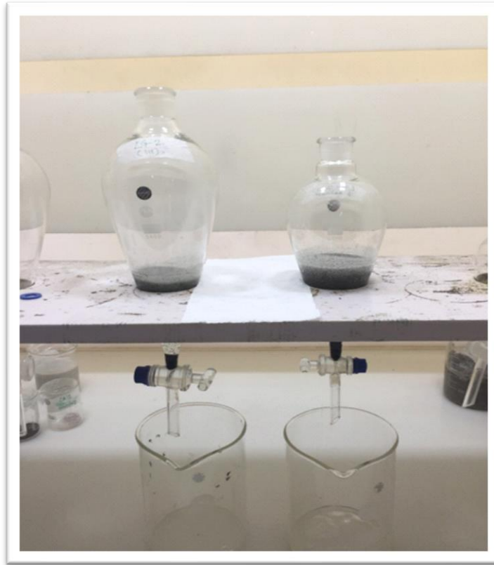
Figure 1.8. Heavy Mineral Separation using separating funnel used for separating heavy and light minerals.
