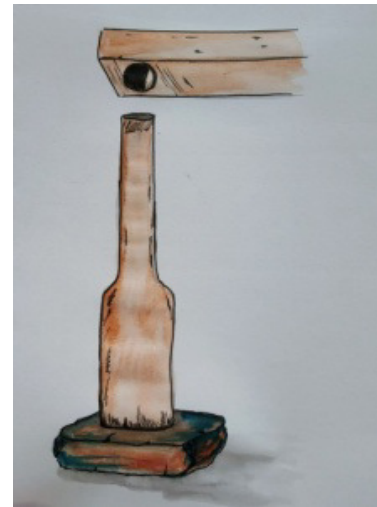
Fig 3.51: illustration of how the posts are put together
