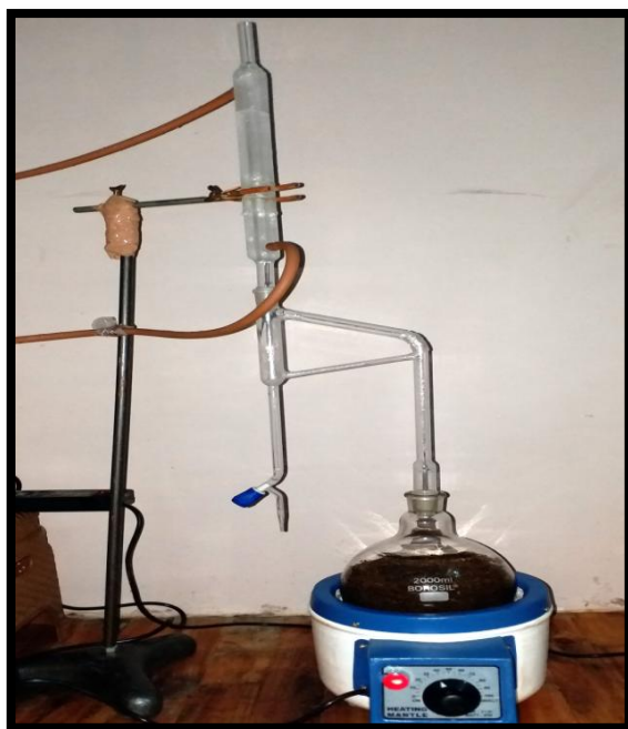
Plate No.21: Hydro distillation by Clevenger apparatus
