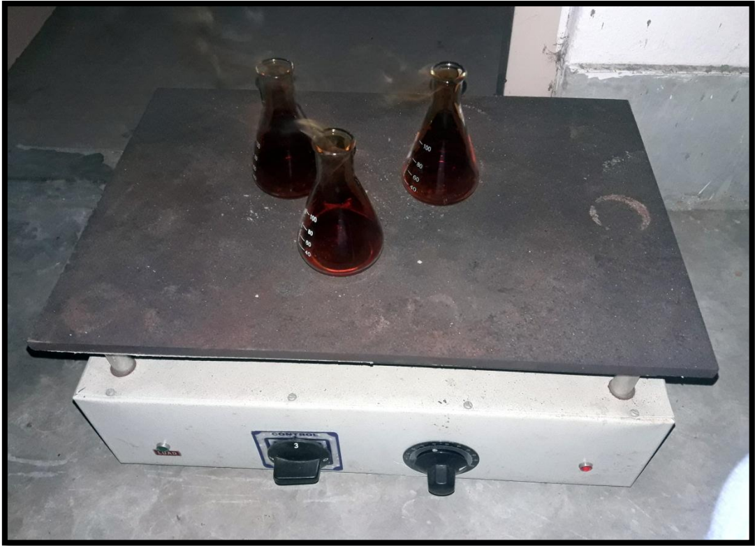
Plate No.34: Open air digestion on hot plate
