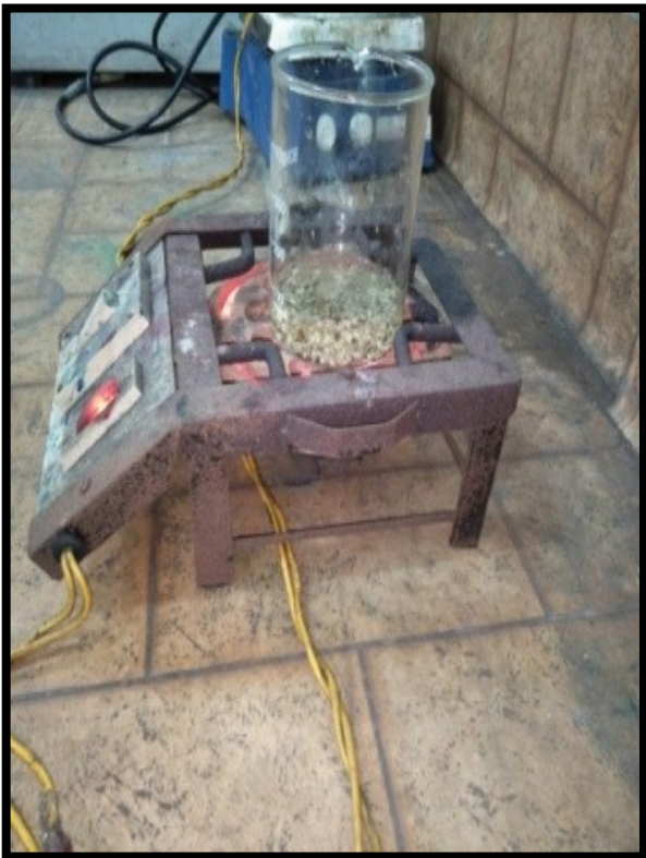
Boiling of peel with citric acid solution
