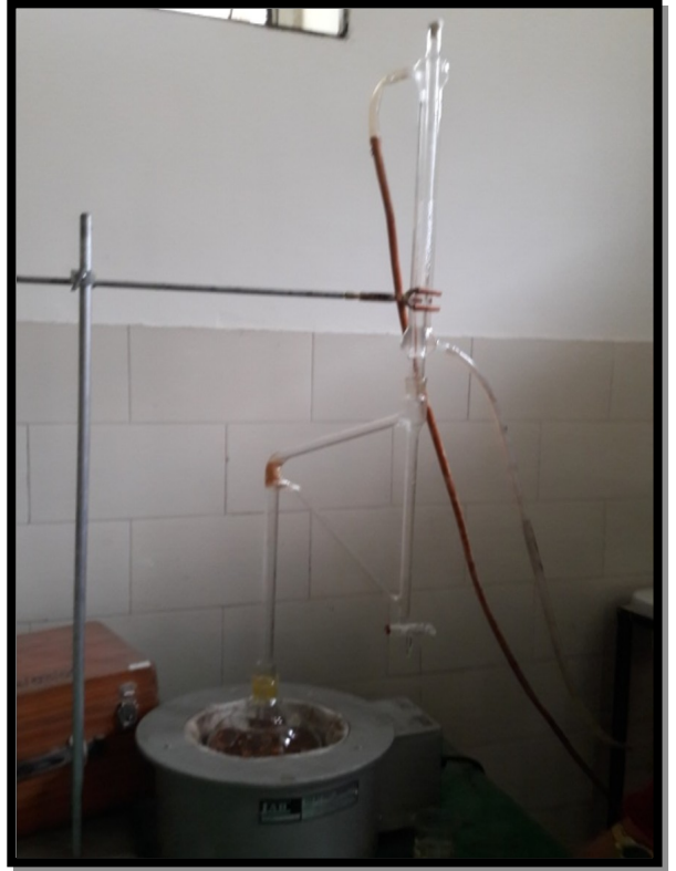
Hydro distillation by Clevenger apparatus
