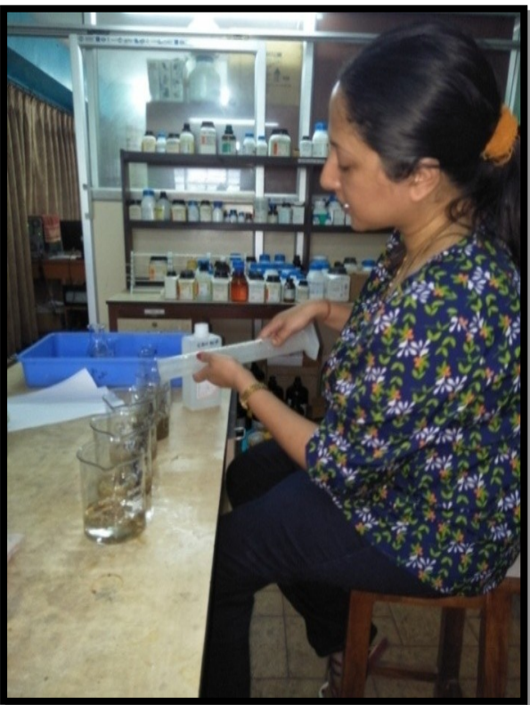
Preparation of sample for open air digestion
