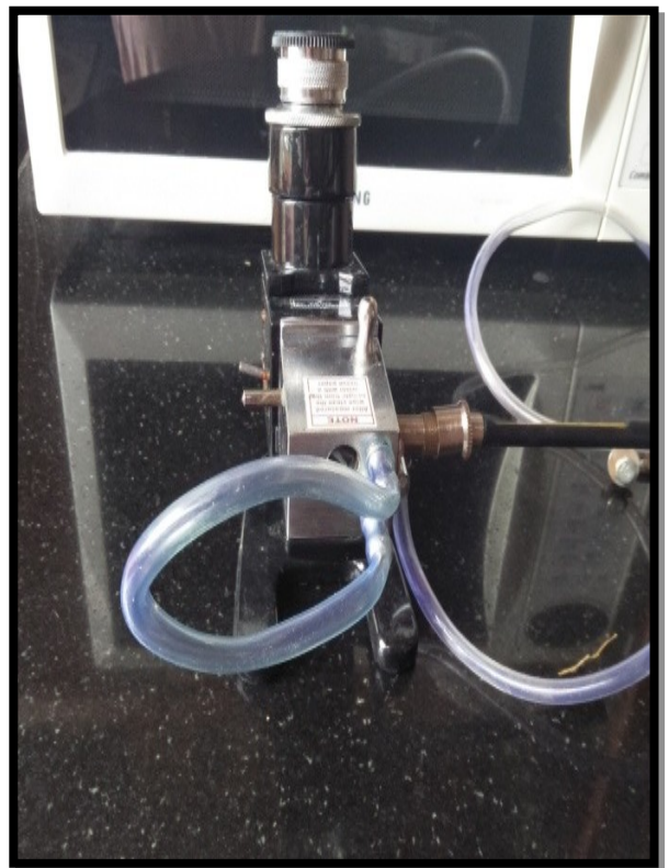
Refractive index determination of essential oil
