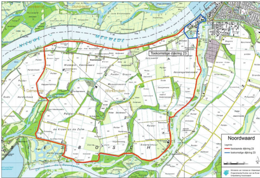
Fig. 4 Future dike ring 23. Existing ring in red; future ring in blue. Courtesy of Source Ministry of Transport, Public Works and Water Management, and Room for the River programme office, 2010. Toelichting Rijksinpassingsplan: ontpoldering Noordwaard. p. 27; released under a Creative Commons Attribution-NonCommercial-NoDerivatives 4.0 International License
