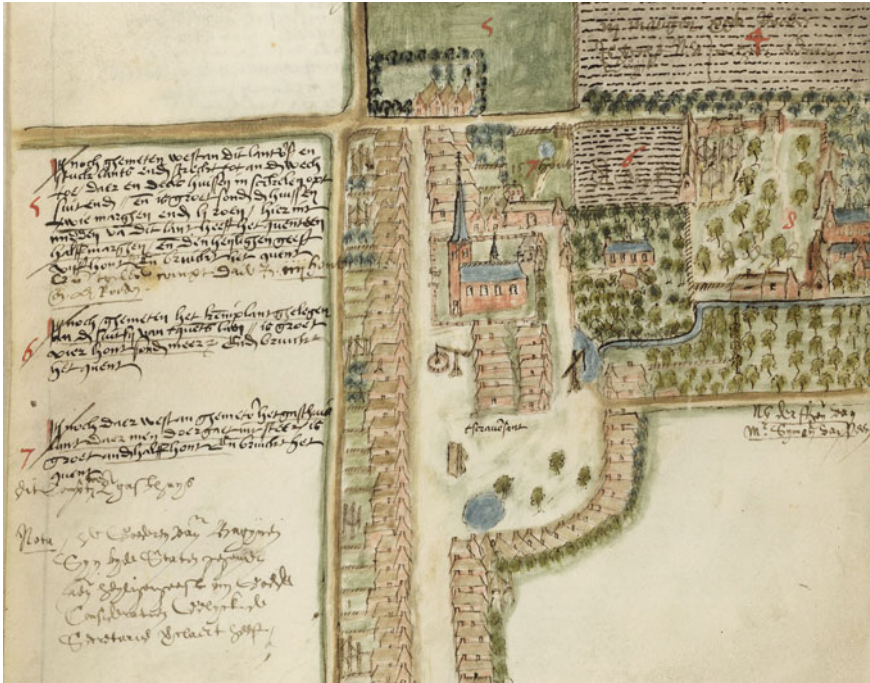
Fig. 7 Detail of map of the town of 's-Gravenzande by Coenraet Oelenzn (1566) with clearly visible public stadswaterputten (wells operated and constructed by the city councils for its inhabitants) with sweeps. One sweep was located near the harbor, and drinking pools providing both ground and surface water to its inhabitants. Source Nationaal Archief; released under a Creative Commons Attribution-NonCommercial-NoDerivatives 4.0 International License
