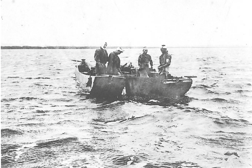
Fig. 3 Fisherman in the Hachirogata lagoon at the beginning of twentieth century. A specific point of the fishing boat is that the boat's bottom is flat because of the shallow water of the lagoon. Source The Fisheries Experiment Station of Akita prefecture, "The report on the using the water area of the Hachirogata Lagoon; 八郎瀧水面利用調査報告書," Akita Prefecture, 1916; released under a Creative Commons Attribution-NonCommercial-NoDerivatives 4.0 International License
