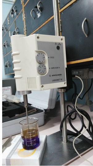
Figure 3.2: Ultrasonication of C_{70} using LABSONIC-M homogenizer.
