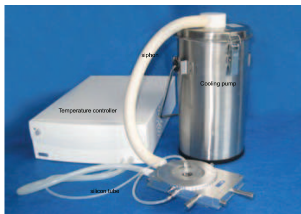
Figure 3.10: LNP95 liquid nitrogen cooling pump connected to THMS600 stage
