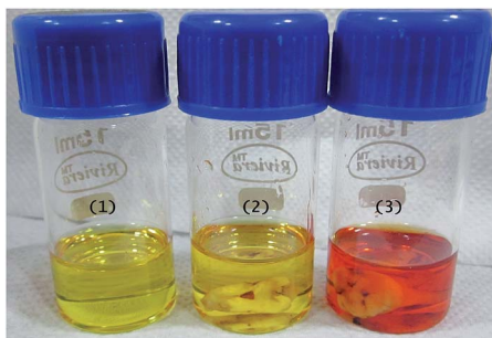
Fig. 4 Colorimetric detection of F^- from fluorosis affected tooth sample: (1) 1 \times 10^{-4} M DMSO solution of L ; (2) L remains silent with non fluorosis tooth sample; (3) after dipping the fluorosis affected tooth sample into the DMSO solution of L for 5 minutes.
