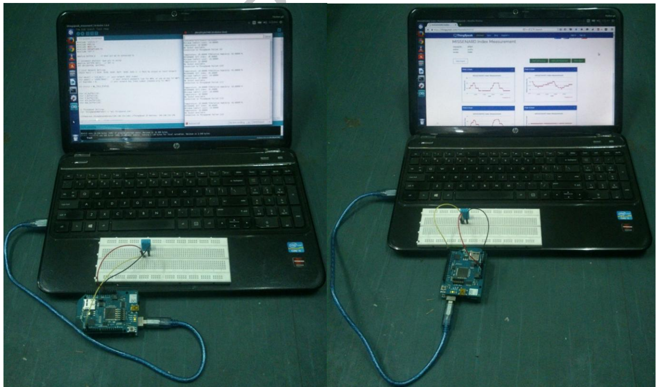
Fig. 6. Experiment set up for IoT based MISSENARD index measurement. Code running on IDE and serial monitor output (left), ThingSpeak cloud running (right).
