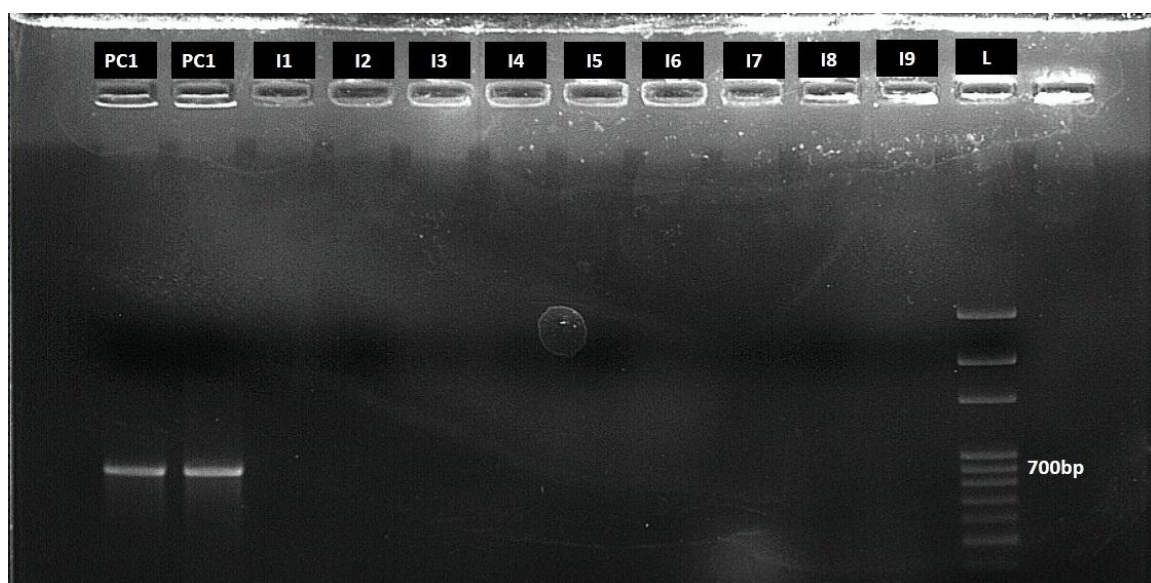
Fig.31c. mecA gene (679bp), PC1/2- Positive Control, L= 100bp Ladder, I= Isolates, I1-XTR1, I2-17R2, I3-XTR10, I4-YTPR1, I5-TY1, I6-AYN2, I7-TP12, I8-BPP1, I9-TB9.
