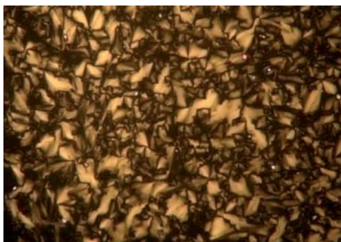
Fig. 2 Representative POM image of [C_{16}VIm]I at 100\text{ }^{\circ}C .
